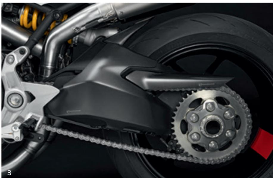
2\_Adjustable Öhlins steering damper. 3\_Carbon swingarm cover.
