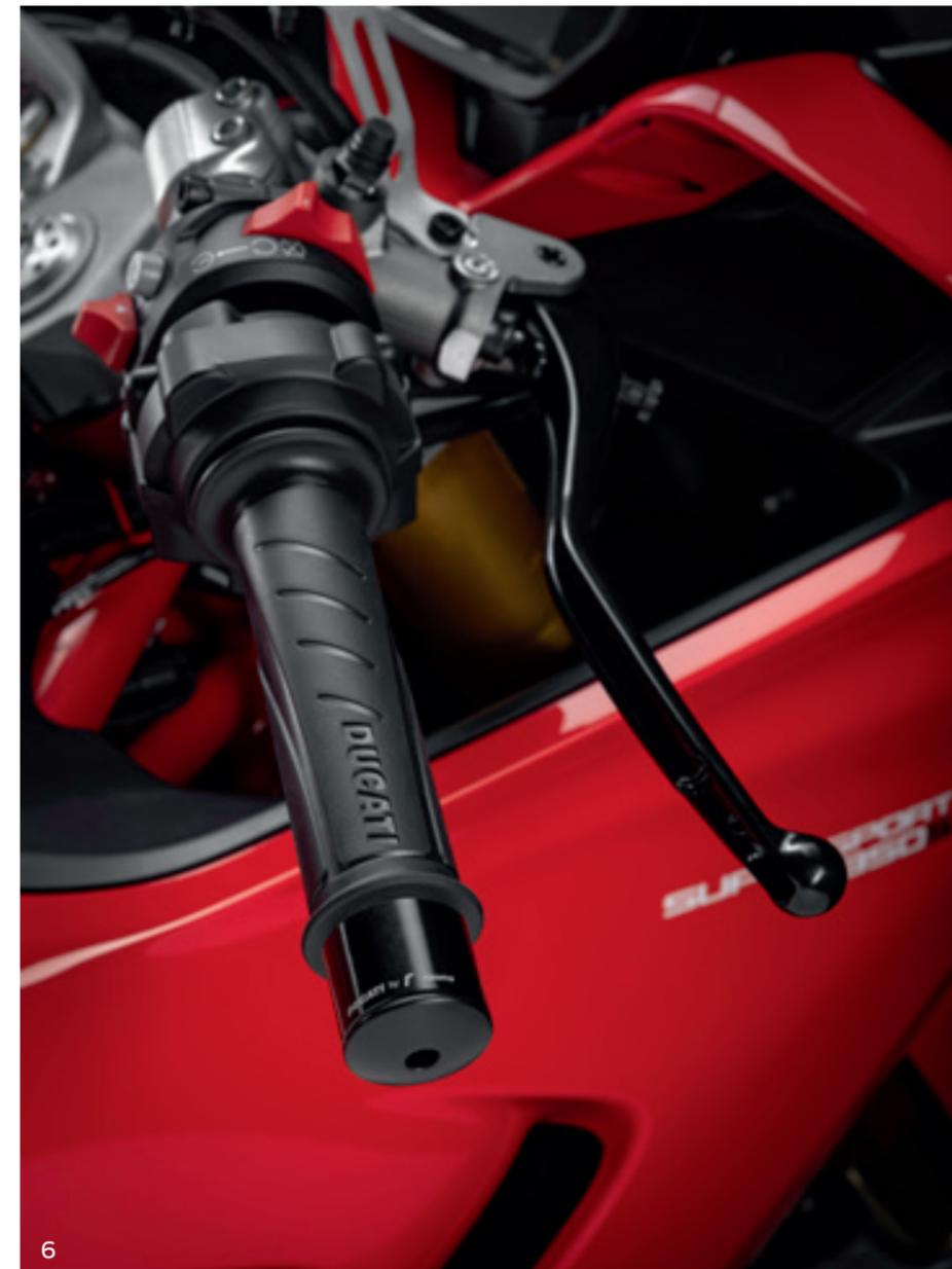
5\_Silencers. 6\_Billet aluminium handlebar counterweights. ■ ■ ■ A
