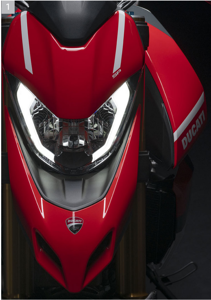
1 Headlight with Day Time Running Light (DRL)
