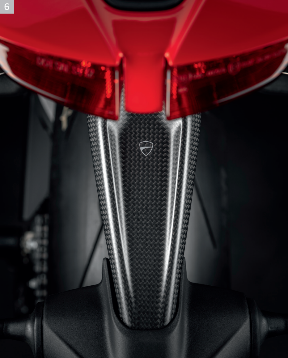
6 Carbon number plate holder support
